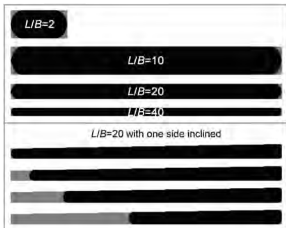
Fig. 11 Detachment of flat-ended stamps with rectangular cross-sections having various aspect ratios L/B . We show only the final stable states. Independently from the aspect ratio, the final state corresponds to almost complete rectangle with rounded-up corners. When the shape has an inclination, a continuous detachment becomes possible.
