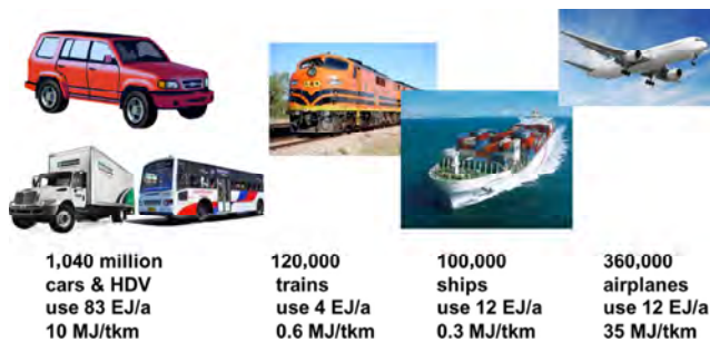
Fig. 6 Number of transportation vehicles worldwide and their global annual energy consumption and energy intensity (energy consumption per tonne weight transported and kilometre).
