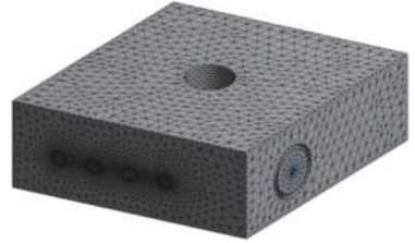
Fig. 6 Thermal-flow-solid coupling finite element model
