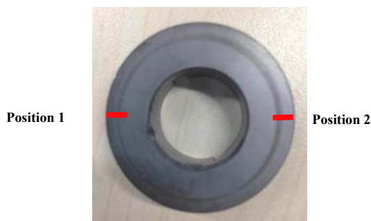
Fig. 8 Position of wear track depth measurement 图8 磨痕深度测量点示意图
