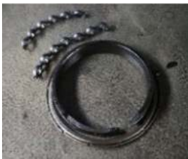
(c) Damaged bearing
